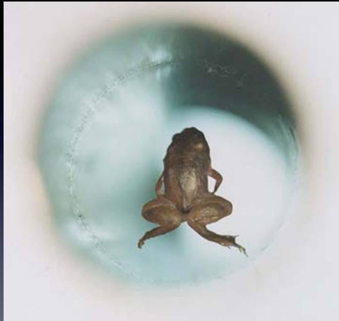
A live frog levitates inside the vertical bore of a Bitter solenoid in a magnetic field
